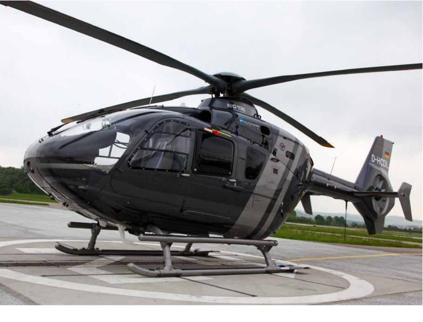
creating one more passenger space or allowing an owner pilot to be up front with a professional pilot alongside. The twin engines allow for a level of redundancy in the event of one engine failing during flight, although this is no guarantee that you will not wind up in the water anyway. The "fenestron" tail rotor, which encloses the tail rotor blades and is unique to Eurocopter, adds a degree of safety to people outside of the aircraft, as well as when manoeuvring in confined areas.
