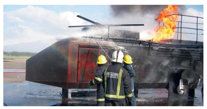
Discrete foam monitors can be installed on the helideck, operated by a push button from the helideck or the bridge. The nozzles can be recessed in the deck itself, so as not to interfere with the obstruction free landing area. A level of redundancy must be allowed for should one or more of the monitors get damaged during the crash. Modern foam systems can be effective with just a 1% foam mix, affording a considerable saving of space and weight.
